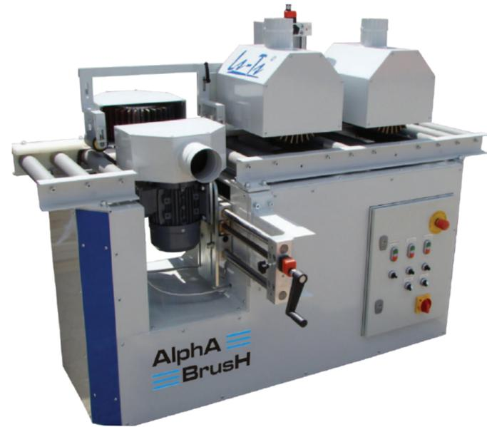
The sanding heads can be mounted on the top (T), the bottom (B) or the sides (S) with as many sanding heads as needed. Standard sanders include the TS, TB, SB or TSB. Custom machines with extra sanding heads are available upon request. Standard machine width is 300mm & parts height 100mm.
